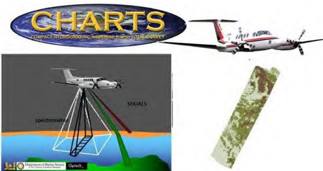
Figure 6-14. USACE GPS-controlled CHARTS hydrographic surveying system (JALBTCX)
